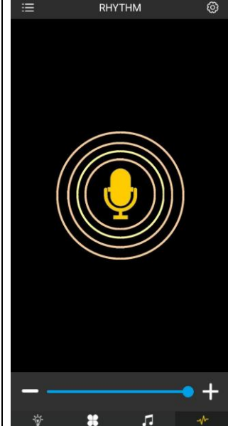
This section of the app activates the phone's microphone. The lighting follows the rhythm of the sound. The sensitivity can be adjusted.
